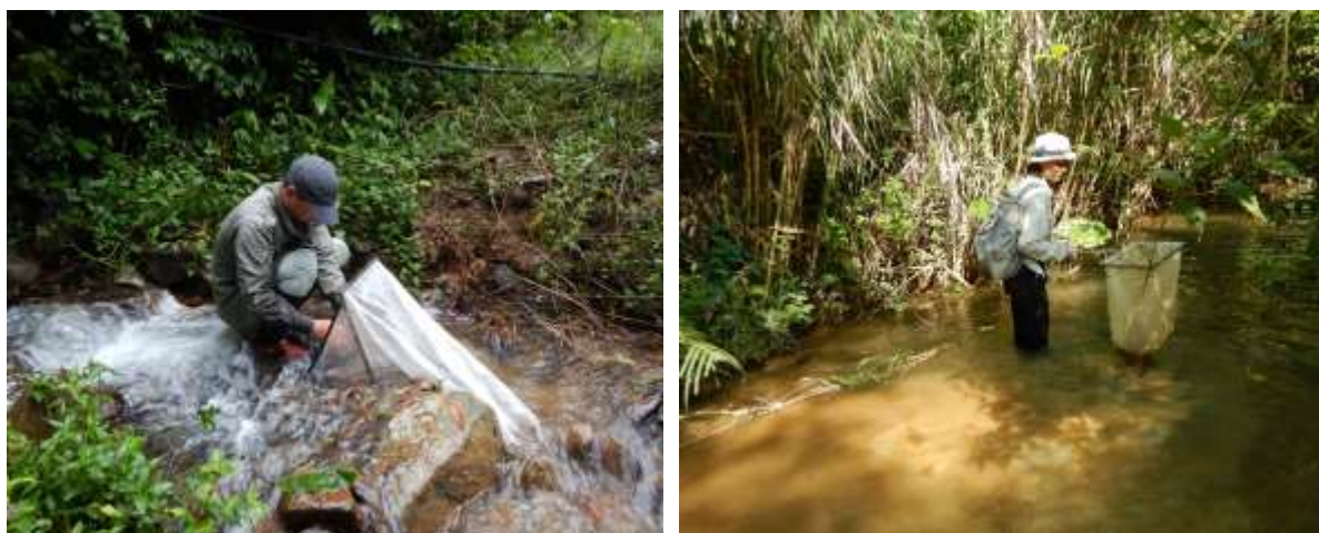
a) Collecting sample by Surber Sampler
